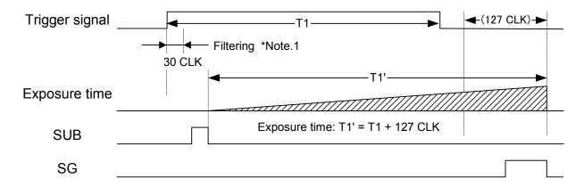
Notes: The trigger signal equal to or shorter than 30 CLK is removed by the filtering system.
